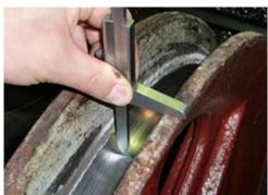
Vernier depth gauge 0-150mm
